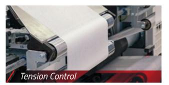
Web Tension is important to monitor in order to maintain consistency in your process. Power/mation installs systems to receive constant feedback of dancer arm position, roll diameter, and current web tension to provide predictable positioning, stability, and web control. Variable Frequency Drives (VFDs), servo motors, induction motors, and peer-to-peer communication setup is also available from Power/mation.
