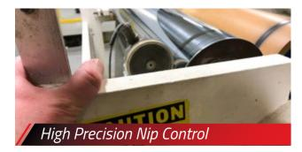
Nip control is important in any laminating and printing application. When you combine our compact, high force electric actuators and linear encoders you will yield a better product and reduce waste. Power/mation can implement these highly accurate closed loop systems to gain better control of your nip.
