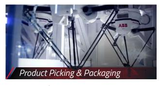
Picking product from a moving conveyor and placing them into a container can be a challenging application. PickMaster® Twin is the market-leading robotic software for vision-guided random flow picking and packing. Integrating conveyor tracking and vision cameras into one solution allows flexibility for many applications.
