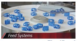
A flexible feed system that works through combining actuation of servomotors and an impulse generator. Once bulk components lie on feeder surface with the right orientation, the vision system can locate them and send coordinates to the robot for pick up. Product changes can be made in a matter of seconds without any difficulty.
