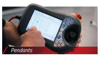
ABB's offering of control pendants is designed to suit both the experienced technician and those who have little to no experience in operating industrial robots. The pendants are easy to use and ergonomically crafted to be comfortable with easily accessible emergency stops.
