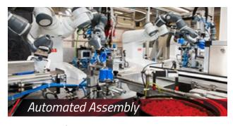
Using robotics for assembly eliminates repetitive tasks allowing personnel to work on more delicate and demanding tasks. Robots can also reduce unwanted repetitive motion injuries and will maximize work cell uptime to increase productivity. You can expect more consistent cycle rates and better product consistency.
