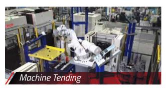
Using robots for machine tending decreases part cycle time, saving you money while ramping up productivity. The process of feeding parts in and out allows the operation to be ready as soon as the current cycle is complete. Using a robot also removes the operator from potentially dangerous work environments.
