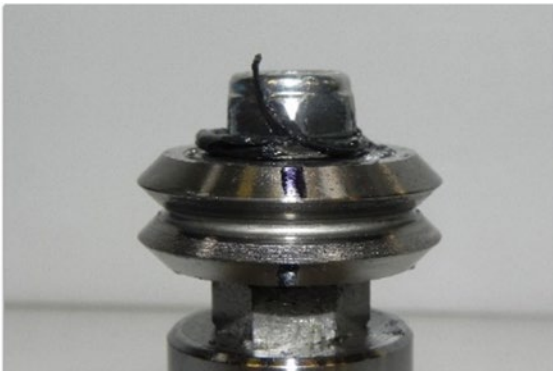
Figure 7. This is a Bishop-Wisecarver guide wheel exhibiting a condition that’s typical for this product line’s mode of end-of-life failure. No shards or fractures are present — and the component is essentially intact.
