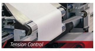
Web Tension is important to monitor in order to maintain consistency in your process. Power/mation installs systems to receive constant feedback of dancer arm position, roll diameter, and current web tension to provide predictable positioning, stability, and web control. Variable Frequency Drives (VFDs), servo motors, induction motors, and peer-to-peer communication setup is also available from Power/mation.
