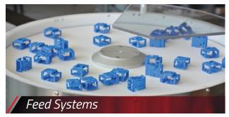
A flexible feed system that works through combining actuation
