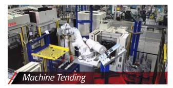
Using robots for machine tending decreases part cycle time, saving you money while ramping up productivity. The process of feeding parts in and out allows the operation to be ready as soon as the current cycle is complete. Using a robot also removes the operator from potentially dangerous work environments.
