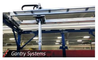
When an application spans a large area, a gantry solution may be the best option. From belt-driven or rack and pinion, to small tabletop or large material handling systems – we have solutions to serve you. Power/mation can provide fully installed systems, or the gantry robot to be installed with your existing control solution.
